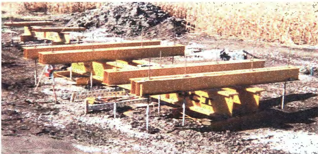
Figure 42. Group load test reaction frame, note individual setup in background
